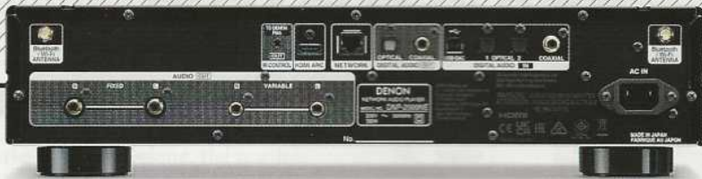
ABOVE: Digital ins include 2.4GHz/5GHz wireless (inc BT) and wired Ethernet, USB-B (384kHz/32-bit and DSD256 as DoP), HDMI ARC, two optical and one coaxial S/PDIF (192kHz/24-bit). Optical and coaxial digital outs are included above fixed and variable analogue outputs on RCAs
