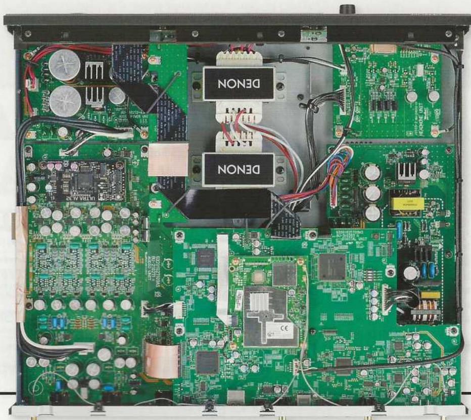
RIGHT: Two mains transformers [top] feed separate PSUs for the wireless/BT PCB [bottom], X MOS and Burr-Brown digital input receivers [bottom right], 'Ultra AL32' DSP [top left] and analogue stage with four ES9018K2M DACs [left]
