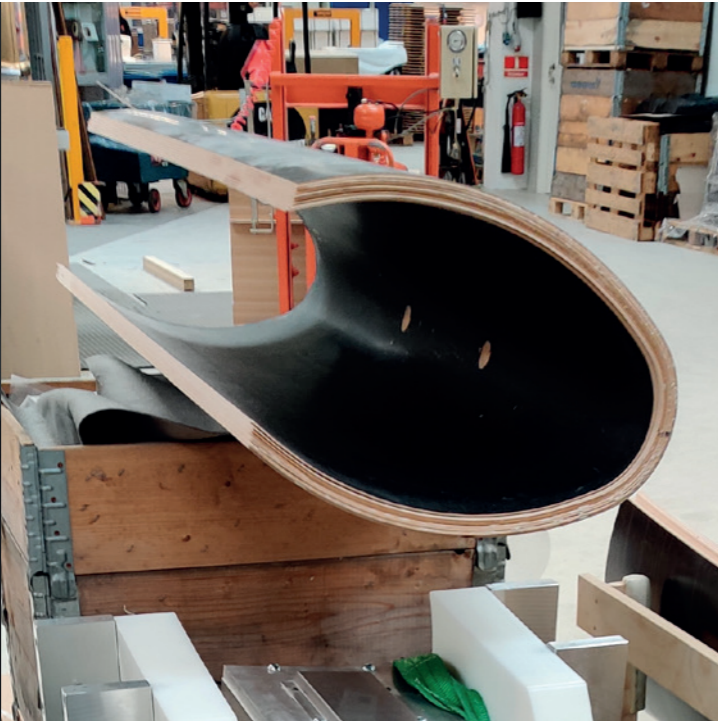
The curved birch laminate enclosure shell is manufactured locally in Denmark. ▽
